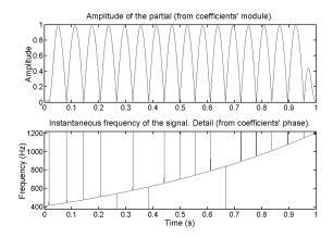
Figure 15: Instantaneous amplitude and frequency of the double exponential chirp.
