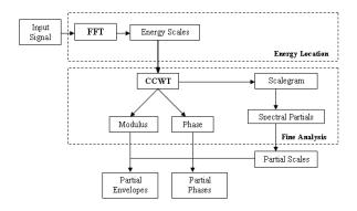
Figure 7: Analysis algorithm block diagram.
