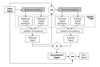
Figure 8: Stationary plus transient algorithm block diagram.
