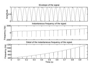
Figure 6: Instantaneous amplitude and frequency of the double exponential chirp signal.
